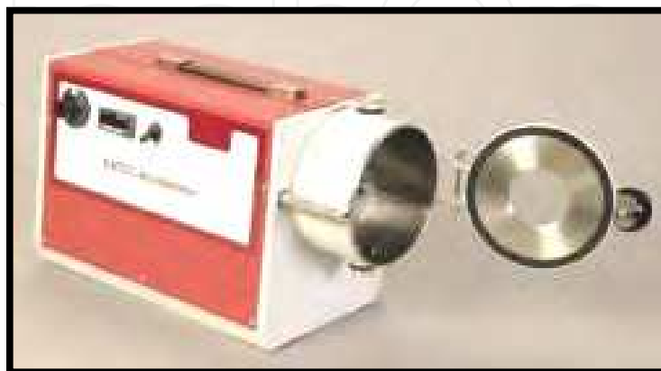
Fig. 8. Accelerator abrasion tester
