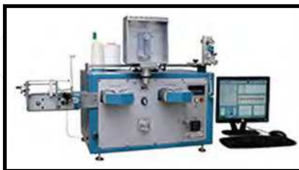
Fig. 11. CTT Instrument with Lint Generation Test Module ( www.lawsonhemphill.com )
