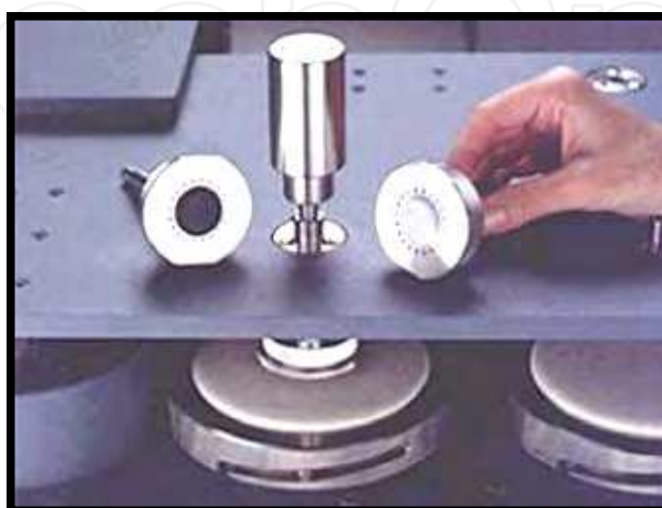
Fig. 16. Setting of sock kit on Martindale apparatus
