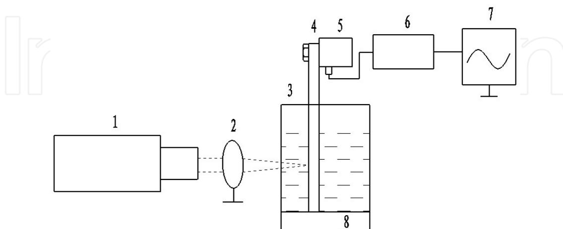
Fig. 5. Schematic diagram of test setup for mechanical effect of laser and metal interaction
