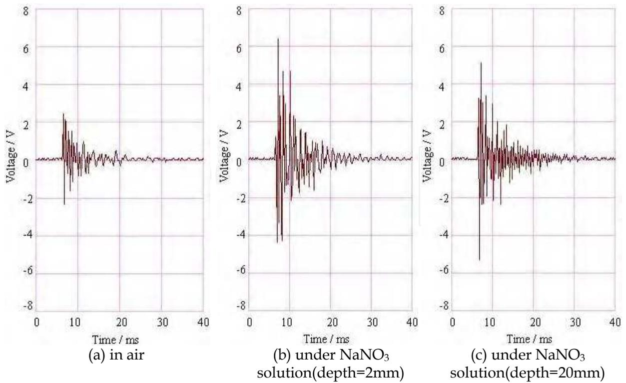
Fig. 7. Mechanical signals of pulsed green laser and metal interaction (150mJ/pulse)
