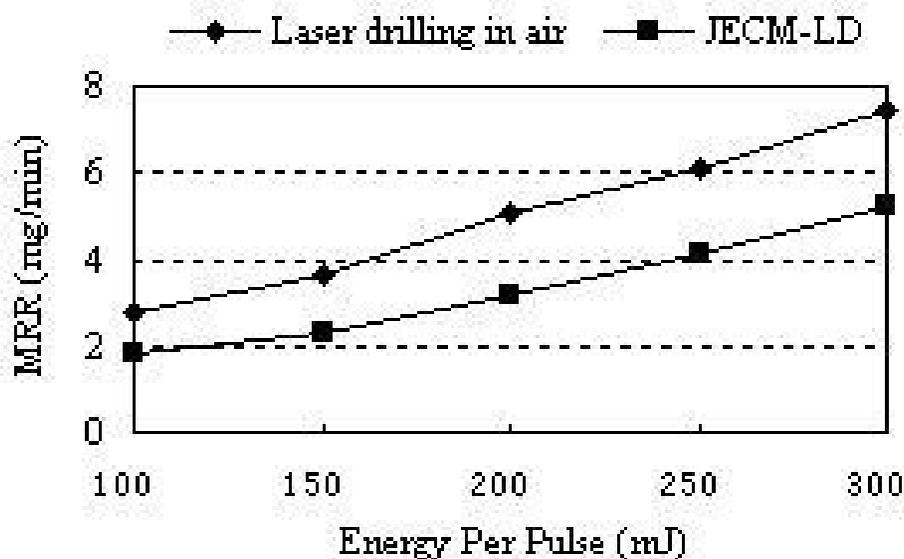
Fig. 19. Effects of energy per pulse on MRR
