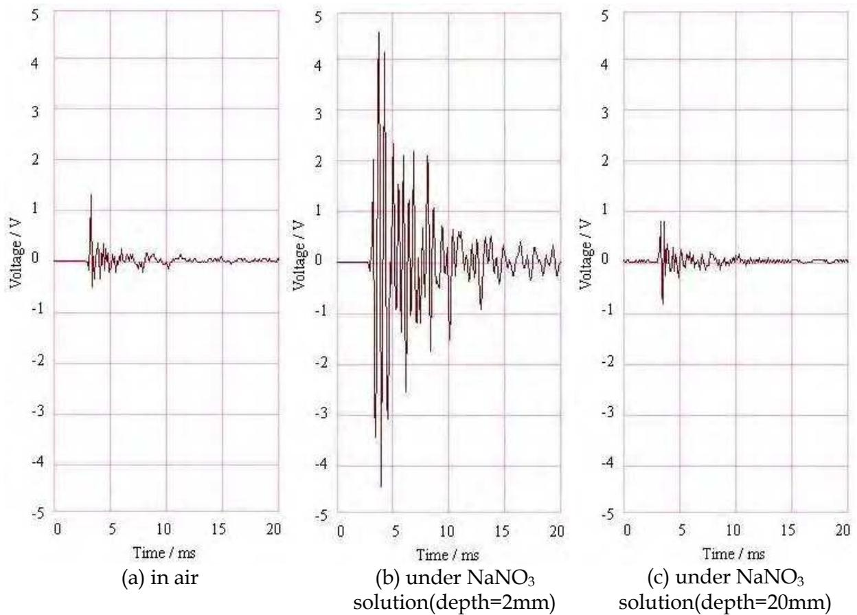
Fig. 8. Mechanical signals of pulsed infrared laser and metal interaction (150mJ/pulse)
