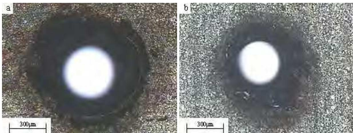
Fig. 15. Micrograph of a penetrated hole drilled with a green laser in air (200mJ, 10s).
