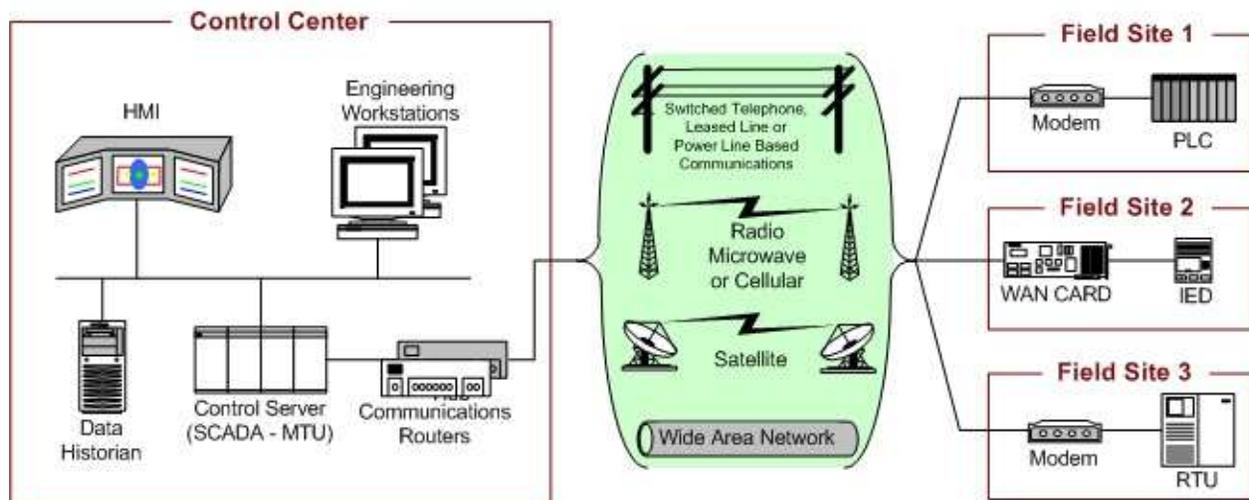
Fig. 2. SCADA sub-systems (Stouffer et al., 2008).
