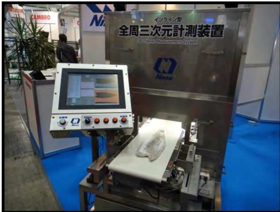
Fig. 11. 3D measurement system that it developed jointly with the National Institute of Advanced Industrial Science and Technology (Anonymous, 2011a.).
