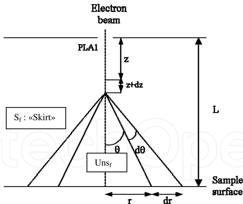
Fig. 4. An electron after PLA1 aperture of the ESEM, moves along the axis of PLA1, undergoes a collision at a distance between  $z$  and  $z + dz$  in an angle of  $\theta + d\theta$ ; it is then scattered and arrives at the surface of the sample in an annulus between  $r$  and  $r + dr$ .
