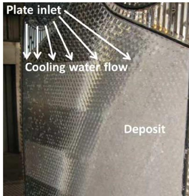
Fig. 5. Deposits formed on the surface of VT-plate.
