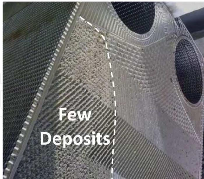
Fig. 8. Deposits formed on the surface of NT-plate.
