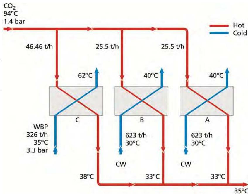
Fig. 4. CO<sub>2</sub> coolers used in the scrubbing process.
