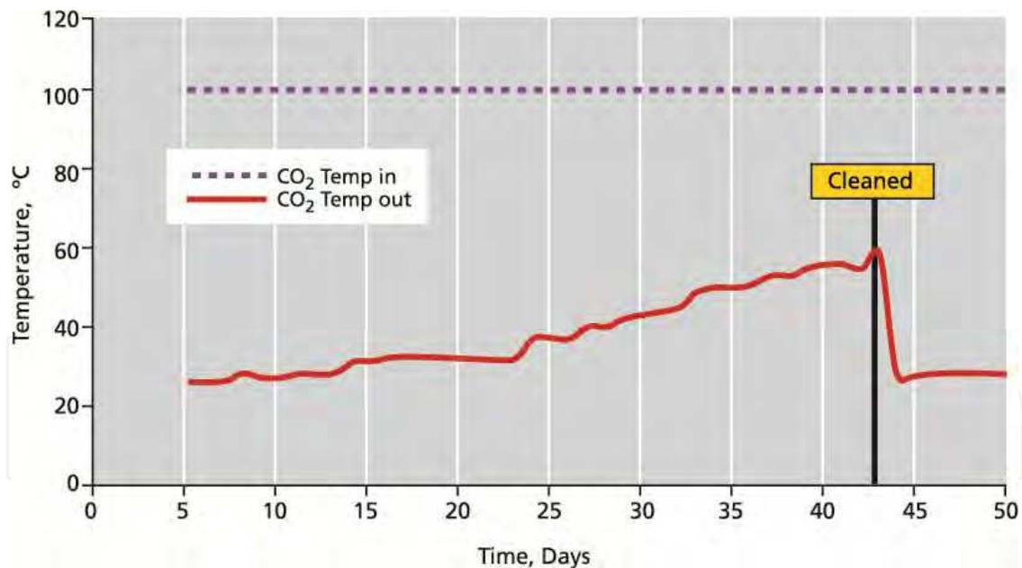
Fig. 6. Inlet and outlet CO<sub>2</sub> temperatures as a function of time.
