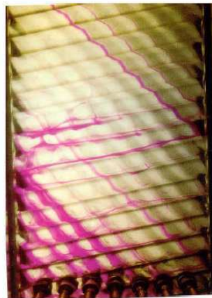
Fig. 11B. Flow visualization by Focke & Knibbe[7], Re=125 .
