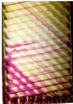
Fig. 11B. Flow visualization by Focke & Knibbe[7],  $Re=125$ .
