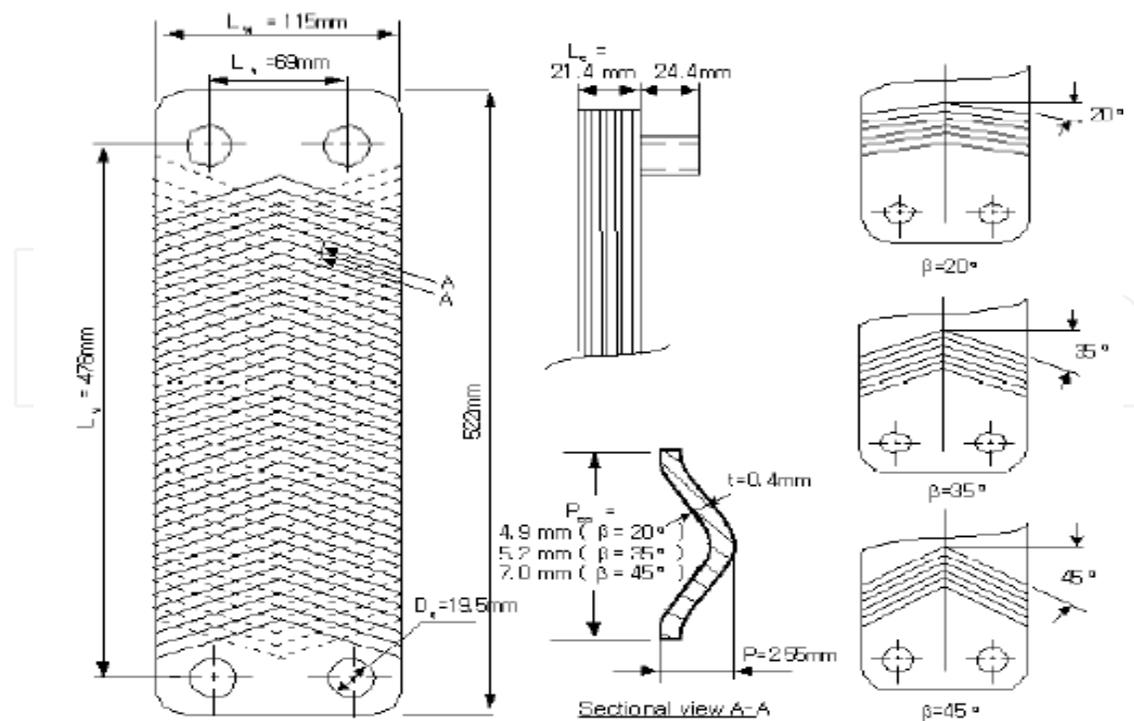
Fig. 2. Dimensions of the brazed plate heat exchangers.
