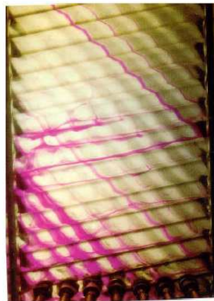
Fig. 11B. Flow visualization by Focke & Knibbe[7], Re=125 .
