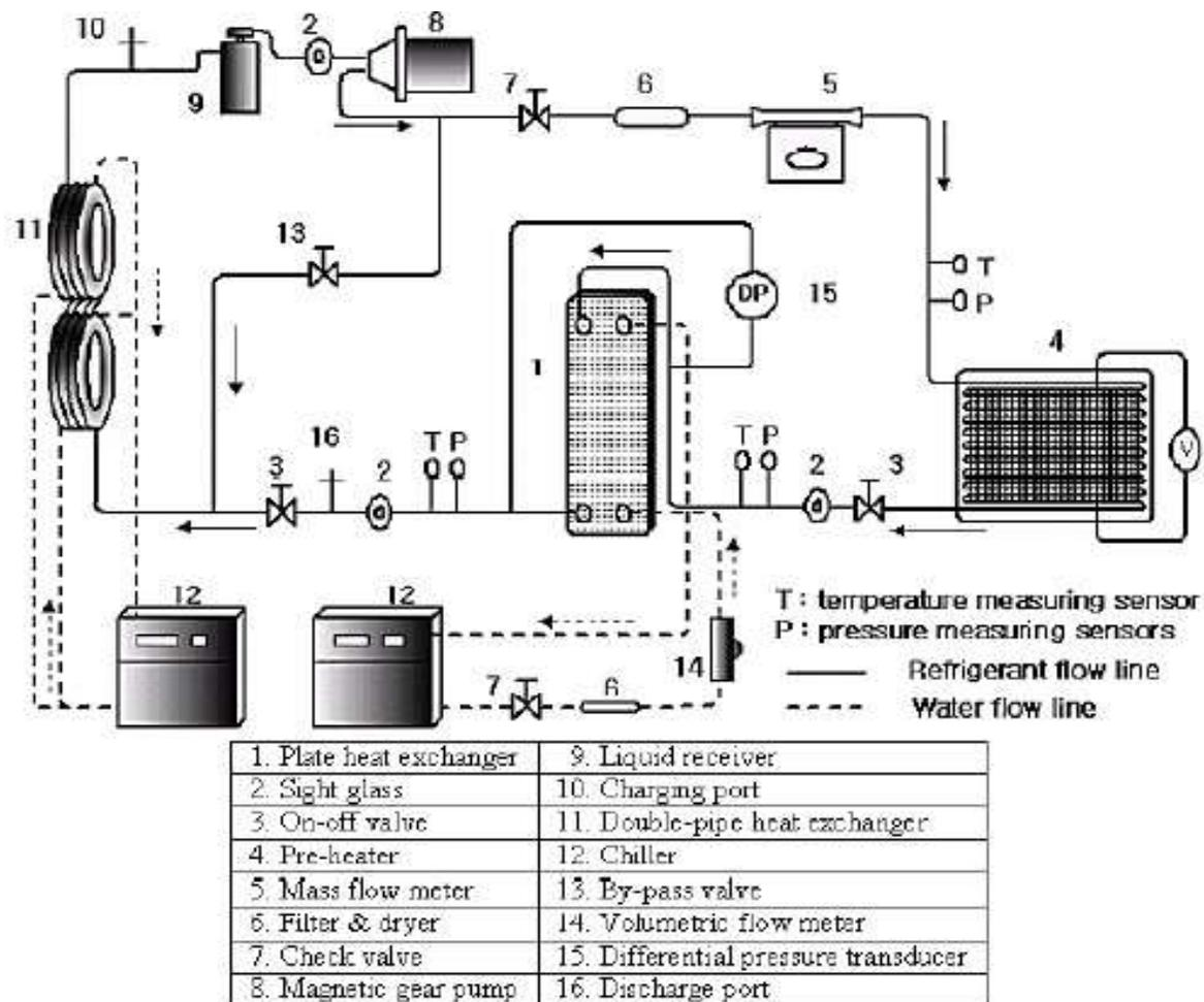
Fig. 1. Schematic diagram of the experimental system.
