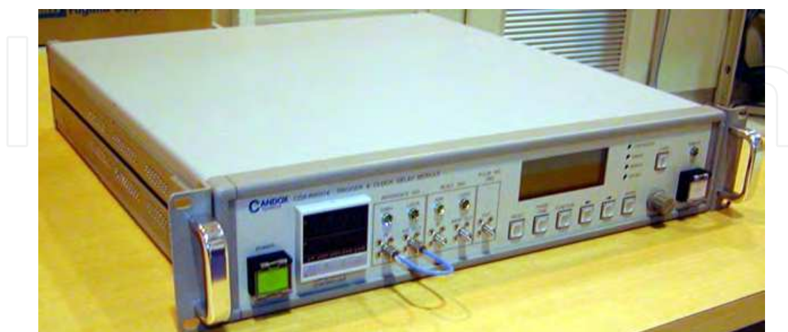
Fig. 6. High precision RF phase control circuit. The circuit provides a delayed RF signal from the output port with a precision of better than 3 ps (in rms) which is independent of the delay time.
