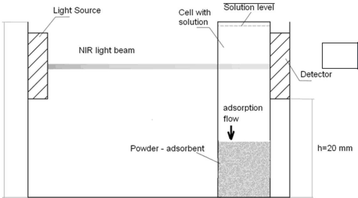
Fig. 1. Experimental setup for measuring adsorption on powders.
