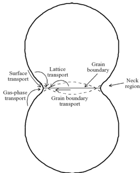
Fig. 3.4. Schematic representation of phenomena involved during firing of ceramics.
