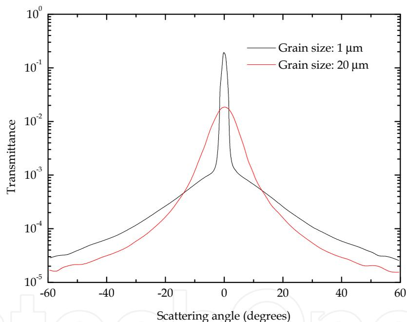
Fig. 4.4. Angular scattering profiles corresponding to 0.8 mm thick polycrystalline alumina samples with  $1 \mu\text{m}$  (solid line) and  $20 \mu\text{m}$  (dotted line) grain size (taken from Appetz & Bruggen, 2003).
