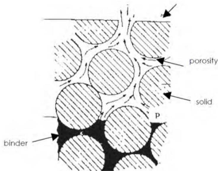
Fig. 3.3. Description of debinding process.
