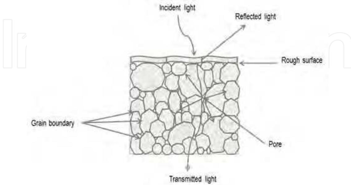
Fig. 4.2. Light scattering sources in polycrystalline ceramics.
