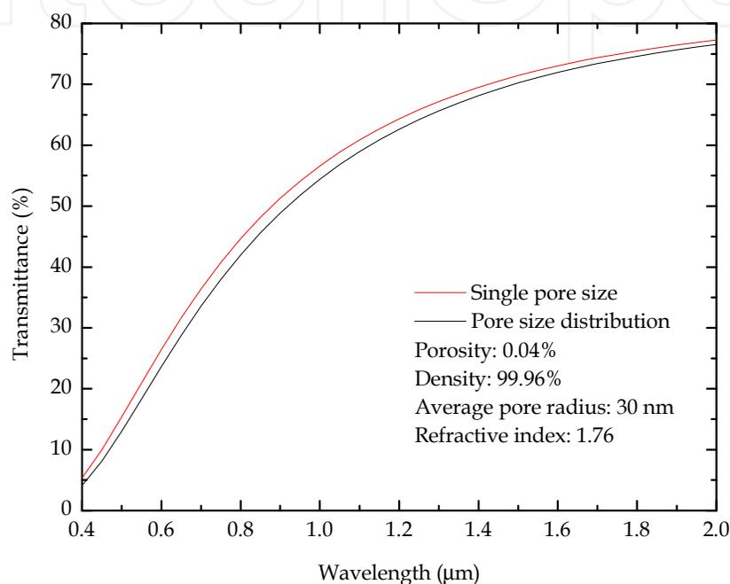
Fig. 4.5. Transmittance spectra in a material with a single pore size or a Poisson distribution of pore sizes.
