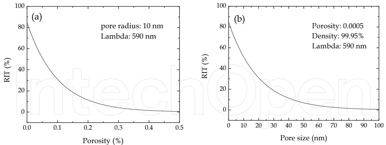
Fig. 4.6. Simulations considering different porosities and pore sizes.
