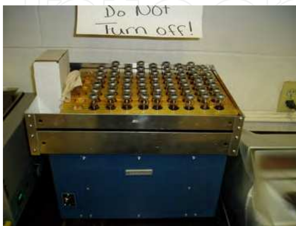
Fig. 3a. Vials shaken to extract MITC.
