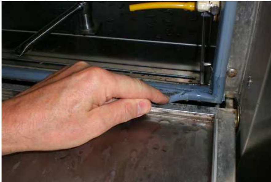
Fig. 4. Damaged rubber gasket in a poorly maintained disinfector used for reprocessing endoscopes. Formation of biofilm in the disinfector resulted in a pseudo-outbreak of Mycobacterium gordonae among patients undergoing bronchoscopy with bronchoscopes reprocessed in the disinfector (Courtesy: Infection Control Team, Odense University Hospital).
