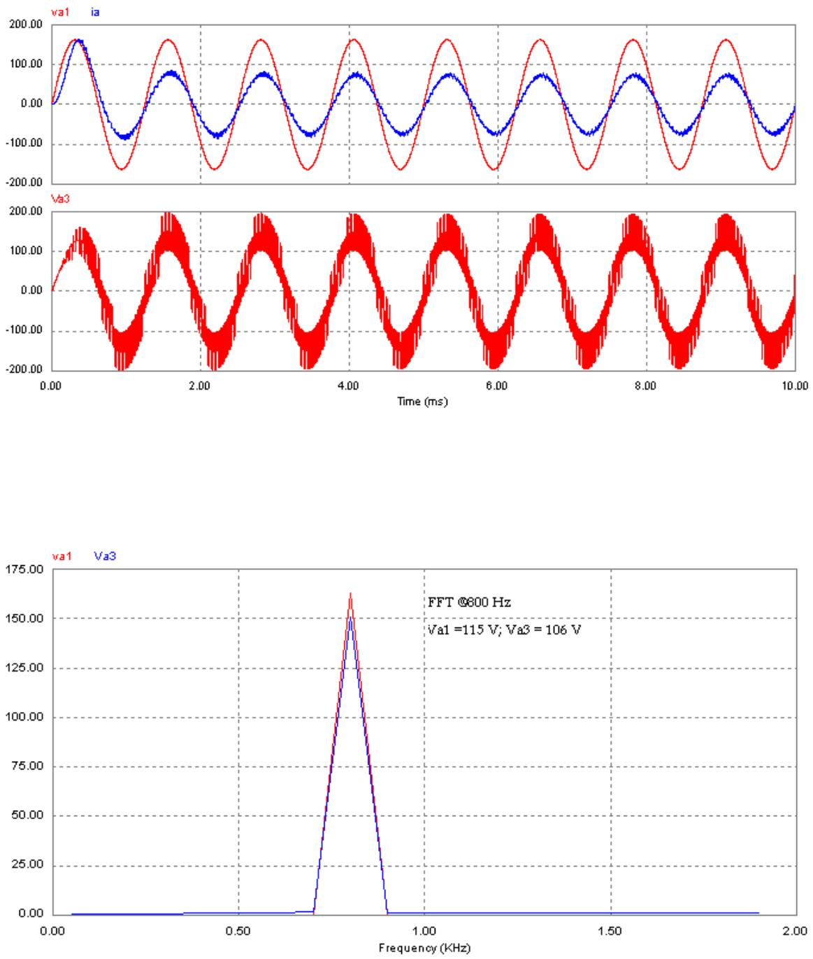
Fig. 22. Results at 800 Hz input frequency for unity power factor.
