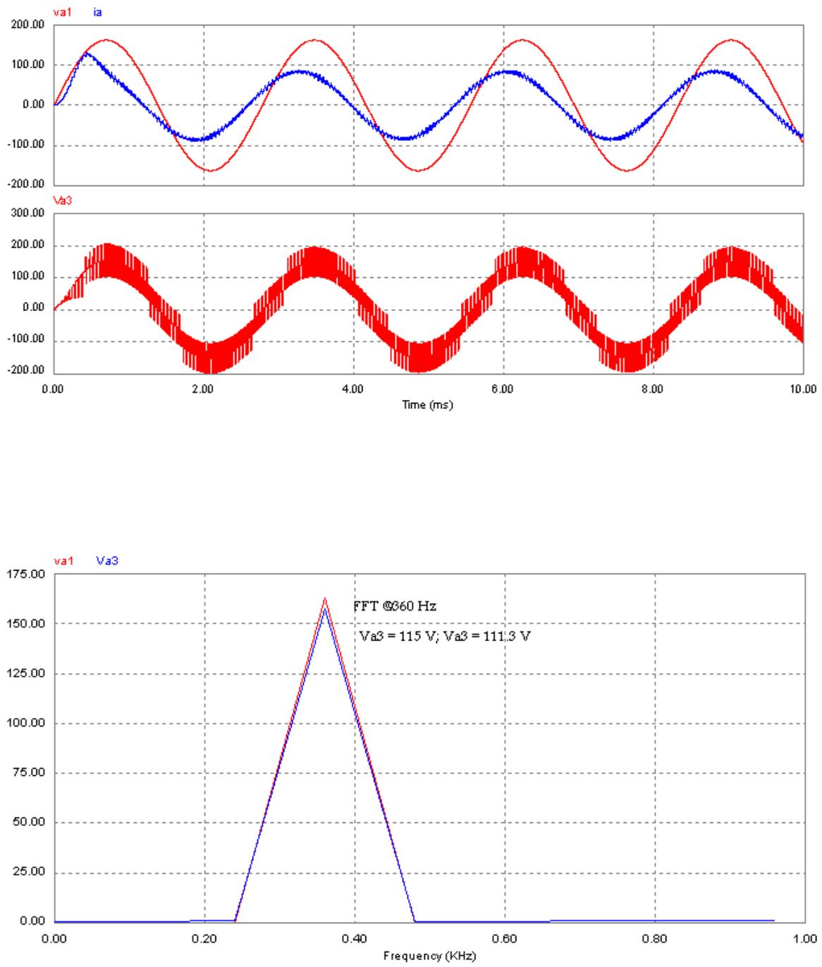
Fig. 21. Results at 360 Hz input frequency for 0.9 power factor.
