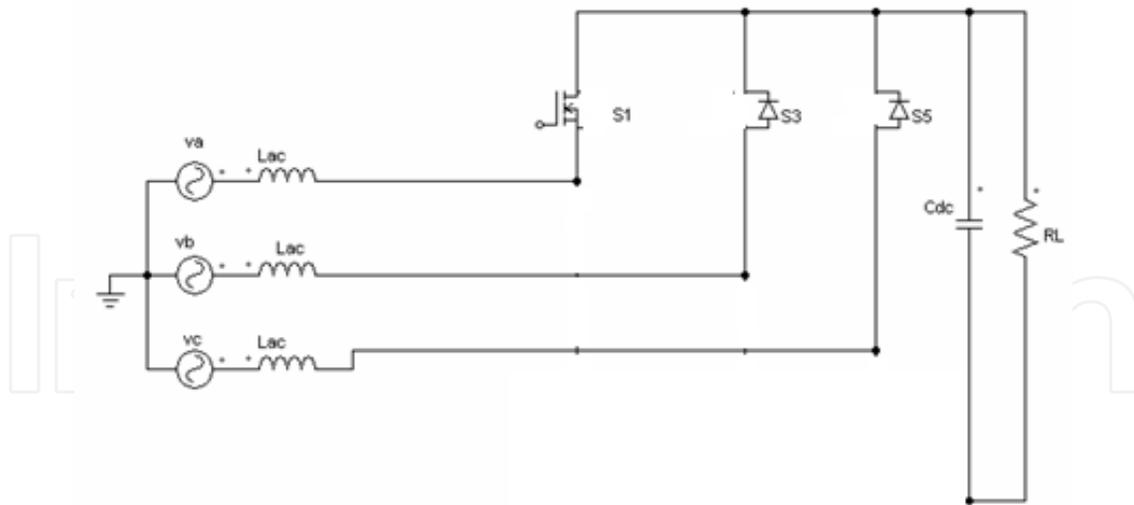
Fig. 3. Boost converter when  $V_a$  is negative.
