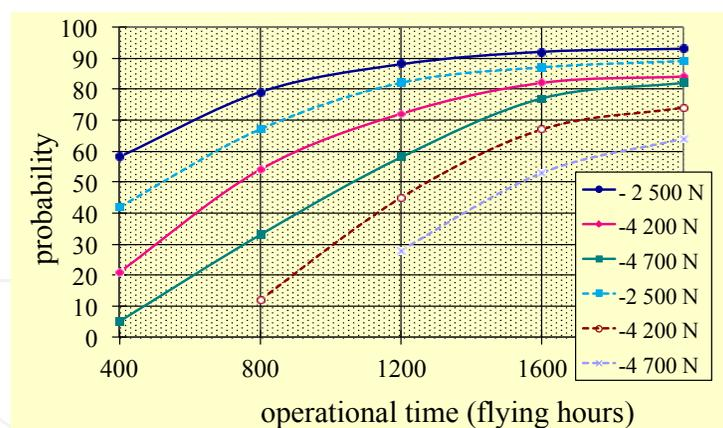
Fig. 5. Probability of lack of generated lift at fighters Mig-21 due to changes in wing geometry during the operation (line - single seat, dot line - double seats aircraft)
