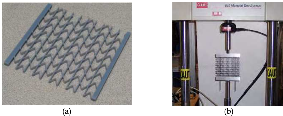
Fig. 11. (a) Example of Objet PolyJet rapid-prototyped zero-Poisson honeycomb, (b) morphing substructure on MTS machine.
