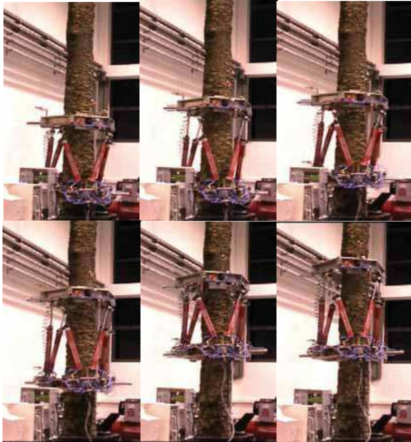
Fig. 5. Different images of the parallel robot climbing o a palm tree trunk.
