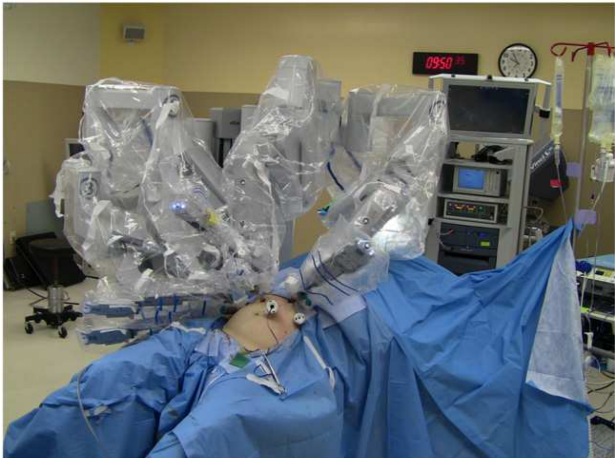
Fig. 2. Robotic platform docked off patient's right shoulder in 10 degree reverse Trendelenburg position, and 10 degree rotation to left.
