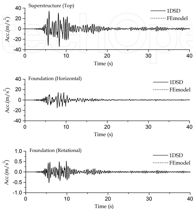
Fig. 9. Time-history response accelerations of superstructure and footing in the horizontal and rotational directions when subjected to ground motion associated with 2004 Ojiya EW by using 1DSDs and the original FE model.
