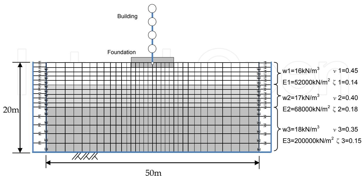
Fig. 4. Two-dimensional FE model for a soil-shallow foundation system supporting a four-story building. The unit weight, modulus of elasticity, Poisson’s ratio, and damping ratio of the  $i$ -th soil layer are denoted as  $w_i$ ,  $E_i$ ,  $\nu_i$ , and  $\zeta_i$ , respectively.
