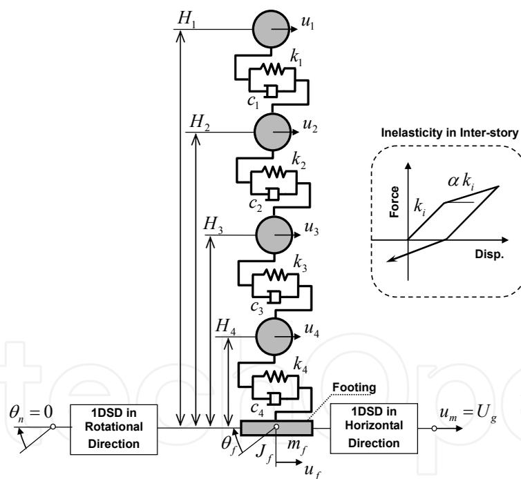
Fig. 7. Numerical model representing complete structural system.
