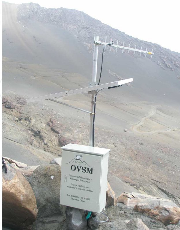
Fig. 1. Seismic monitoring station installed by Observatorio Vulcanológico y Sismológico de Manizales (OVSM) at Nevado del Ruiz Volcano, Colombia.
