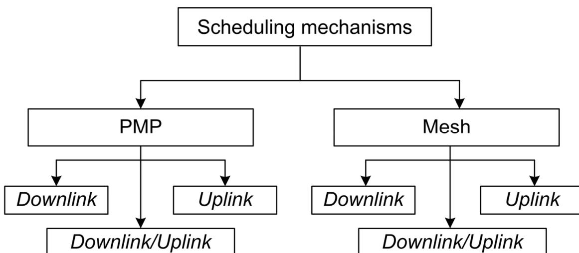
Fig. 3. General classification of WiMAX scheduling mechanisms
