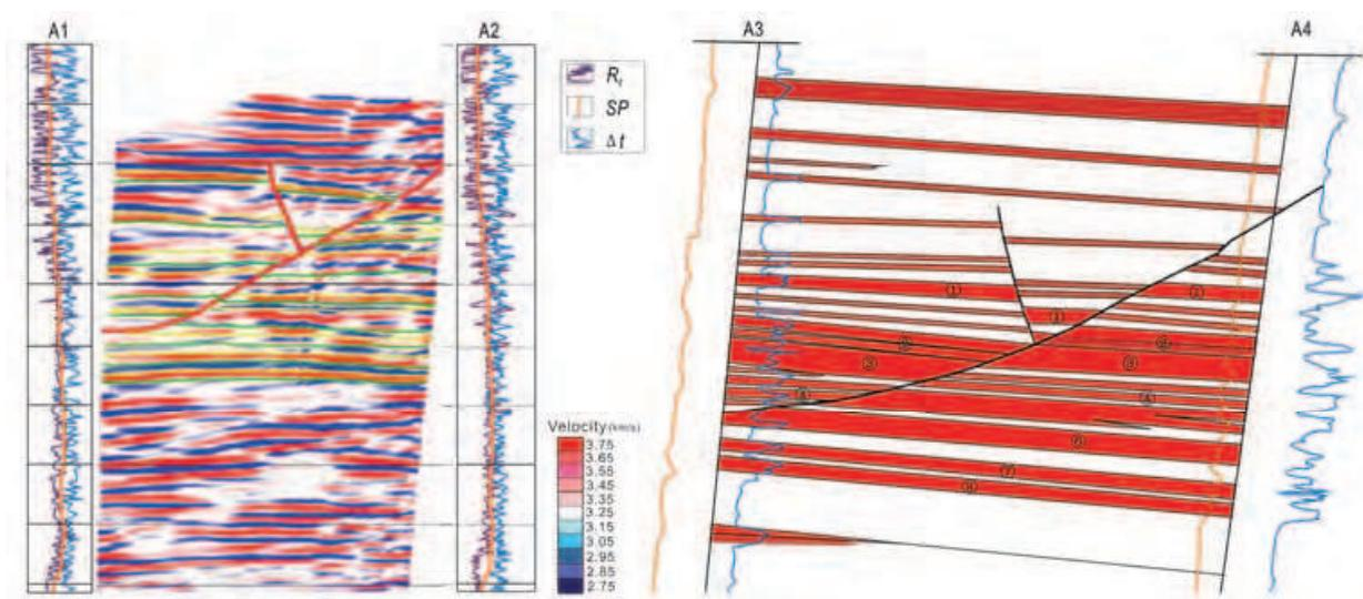
Fig. 4. Application of inter-well seismic survey for reservoir prediction in some oilfield, China. The picture on the left shows the result of interwell seismic imaging and the right one is about interwell seismic interpretation. It illustrates that interwell reservoir heterogeneity can be investigated and small scale faults can be identified clearly.
