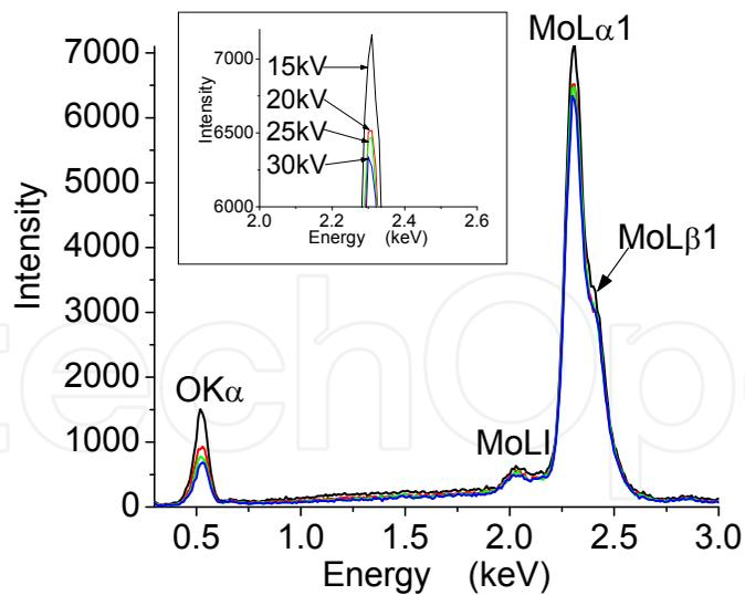
Fig. 2. EDX spectra showing the O and Mo experimental Gaussian peaks at different accelerating voltage. The spectra were obtained under operation conditions of  $T_c=35\mu s$ , DT around 30% and 100s of acquisition time.
