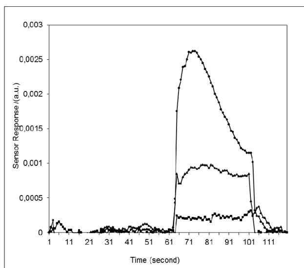
Fig. 1. Sensor response time dependence. (▪) Without laser, (▲) Nd:YAG laser, and (•) CO<sub>2</sub> laser. (Massacane et al., 2010) Permission?
