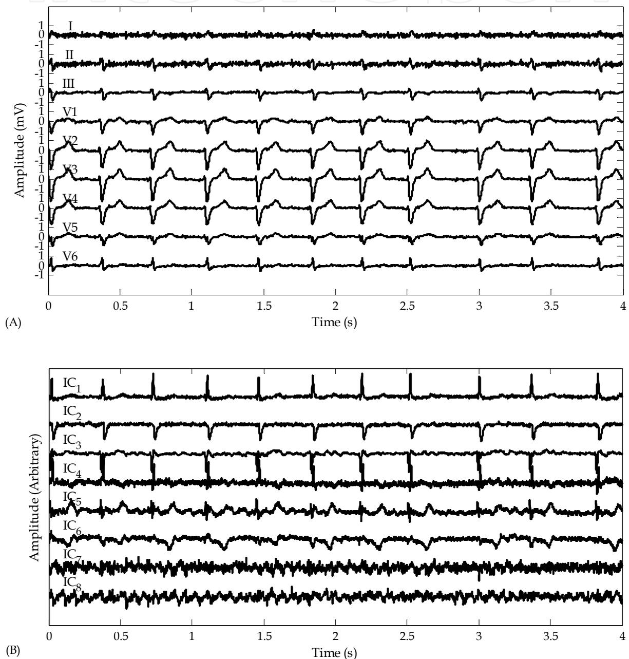
Fig. 6. (A) ECG measured from a patient with atrial fibrillation during exercise stress test. (B) Results of ICA on the signals in (A). Atrial fibrillation is detectable in IC<sub>7</sub> and IC<sub>8</sub>.
