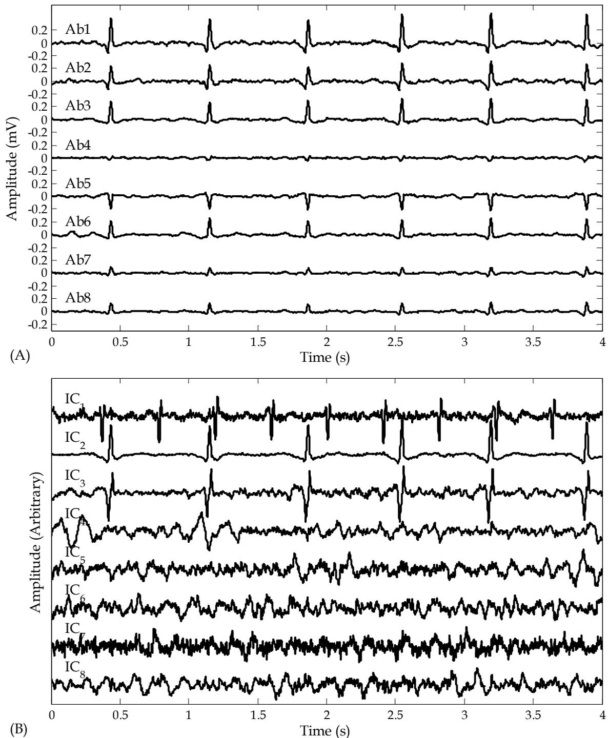
Fig. 4. (A) Eight-lead ECG measured on the abdominal region (leads Ab1 through Ab8) of a pregnant mother<sup>1</sup>. Maternal heartbeats are clearly recognizable but fetal ECG cannot be visually observed. (B) Results of ICA on the data seen in (A). It can be clearly seen that IC<sub>1</sub> exhibits fetal ECG, whereas IC<sub>2</sub> and IC<sub>3</sub> carry maternal ECG.
