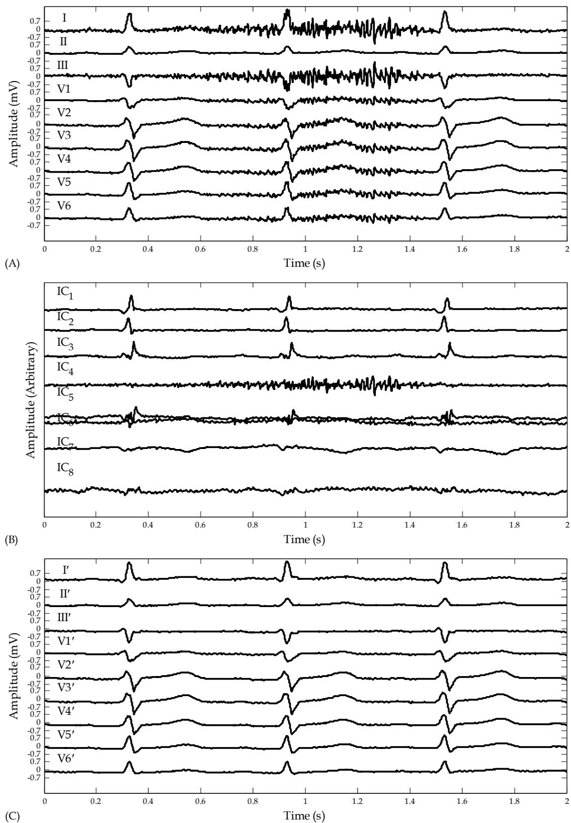
Fig. 3. (A) ECG with left fist clenching artifact visible in all leads but II. (B) Results of calculating ICA on the signals in (A). Fist clenching artifact has been separated into IC<sub>4</sub>. (C) ECG signals reconstructed using all the ICs except IC<sub>4</sub>.
