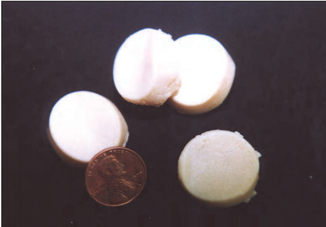
Fig. 8. Recovered “plugs” of precipitated material from Stage I of Three-Phase Partitioning.
