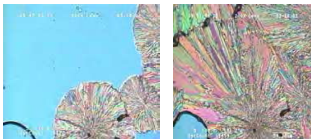
Fig. 10. Spherulites formed upon heating the melt-grown betaxolol hydrochloride.
