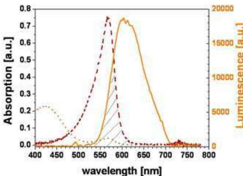
Fig. 10. Luminescence emission spectrum of  $\text{Ru(dpp)}_3^{2+}$  (solid line) and absorption spectra of phenol red in the absence (dashed line) and presence (dotted line) of  $\text{CO}_2$  (20 %). The hatched area indicates the spectral overlap of the donor emission and acceptor absorption.
