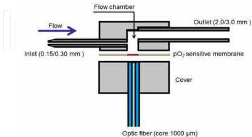
Fig. 3. Schematic draw of the flow through cell
