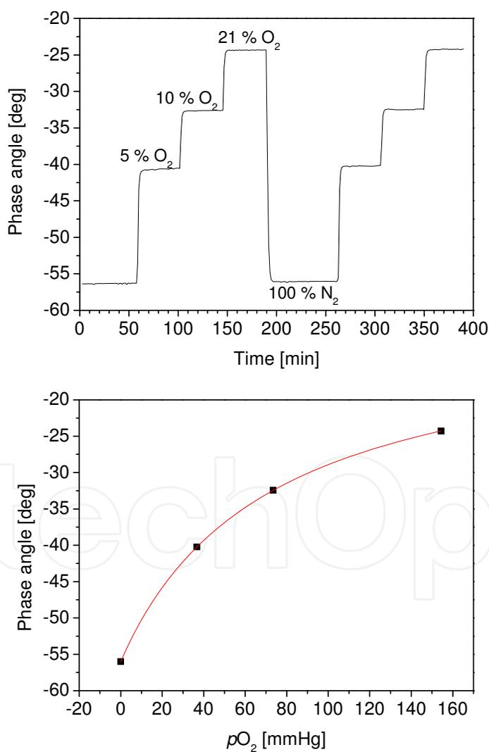
Fig. 11. Oxygen sensor response curve, phase angle as a function of different O<sub>2</sub> concentrations; below: calibration curve obtained by the first cycle of dissolved oxygen concentrations.
