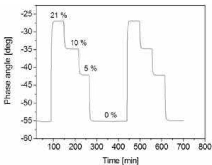
Fig. 5. Example of the experimental protocol used for the characterisation of the miniaturised planar  $\text{O}_2$  sensitive membrane. The measurement is carried out in Ringer solution equilibrated at defined  $\text{O}_2$  concentrations (0, 5, 10 and 21 %  $\text{O}_2$ ) at the constant temperature of 37 °C.
