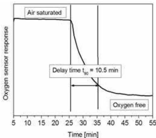
Fig. 6. Measured delay time between 21 and 0 % of O<sub>2</sub> in case of one oxygen sensitive membrane
