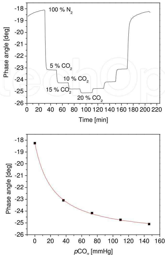
Fig. 12. Carbon dioxide response curve, phase angle as a function of different CO<sub>2</sub> concentrations; below: calibration curve obtained by the first cycle of dissolved CO<sub>2</sub> concentrations.
