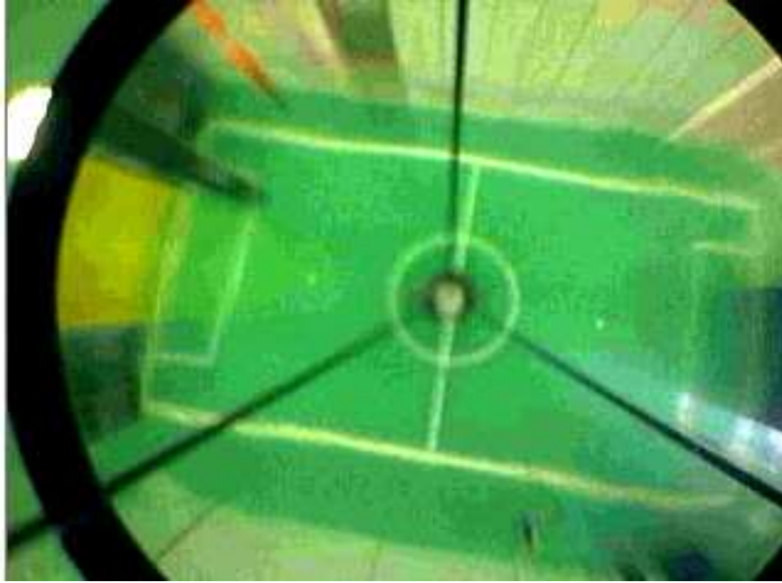
Figure 3. Bird's eye-view of the field obtained by the top catadioptric systems of the robots in Fig. 1
