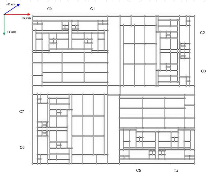
Fig. 9. The extracted IBM POWER4 MCM floor plan
