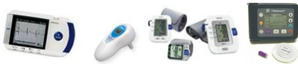
Fig. 1. Omron healthcare products (a) portable ECG, (b) thermometer and (c) blood pressure meter and Philips product (d) vital sense device
