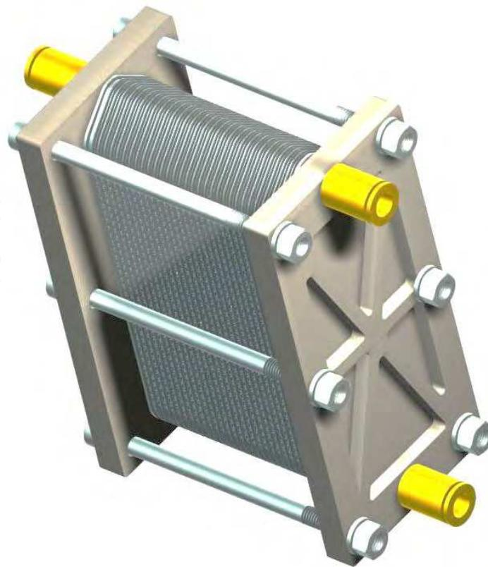
Fig. 2. Schematic design of an air-breathing PEMFC stack
