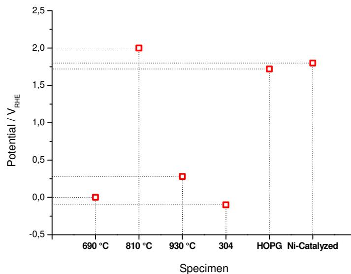
Fig. 7. Corrosion potential of specimen tested in 0.5 M H<sub>2</sub>SO<sub>4</sub> solution at 25 °C [11]
