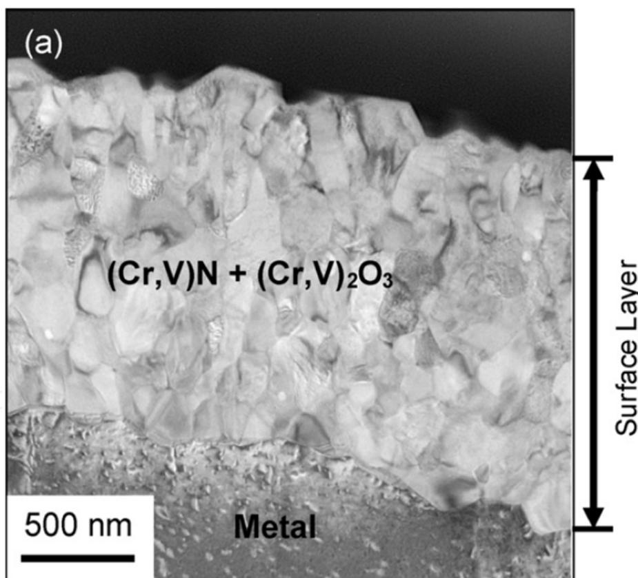
Fig. 8. Microstructures of nitrided Fe-27Cr-6V (850 °C, 24 h, N<sub>2</sub>-4H<sub>2</sub>) bright-field cross-section TEM [87]<sup>3</sup>
