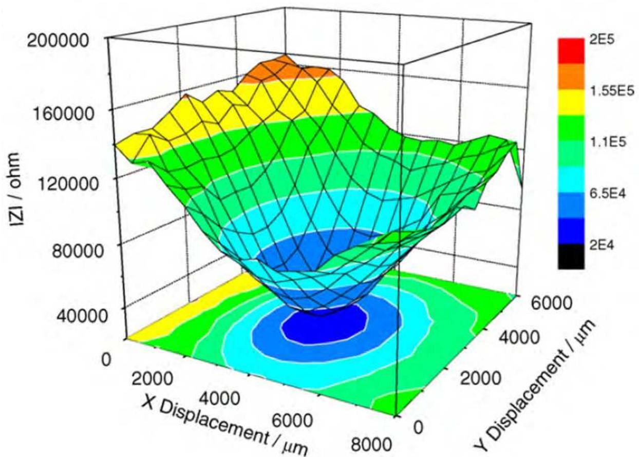
Fig. 14. LEIS maps around the defect [15]<sup>5</sup>
