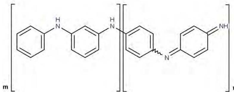
Fig. 11. Chemical structure of Polyaniline (PAni) [7]
