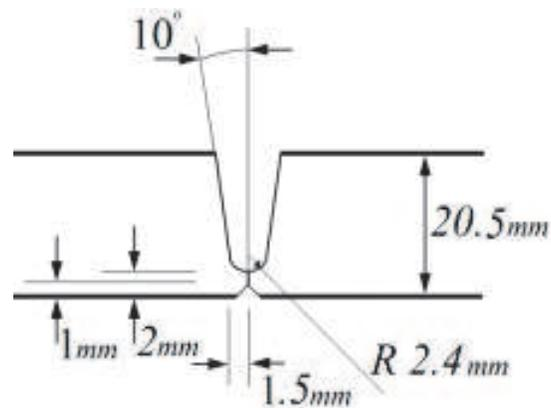
Fig. 6. Joint configuration in the experiments
