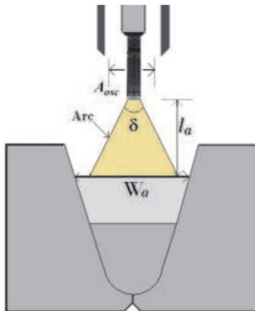
Fig. 3. Seam and arc with nozzle oscillation amplitude
