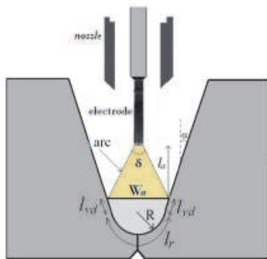
Fig. 1. A schematic view of the arc, melting wire area and seam walls
