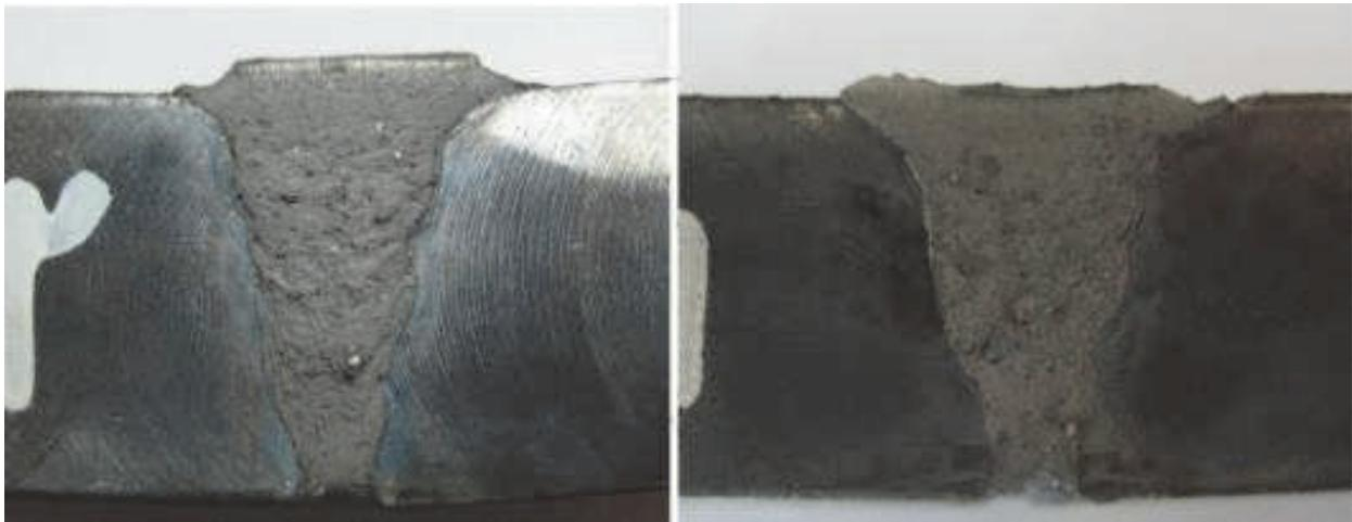
Fig. 7. Front view of the weld sections,  $32.3\text{J}/\text{mm}^2$  WHI and  $393\text{ J}/\text{mm}$  heat input according to *Ex. 1* parameters (left);  $35.2\text{J}/\text{mm}^2$  WHI and  $337\text{ J}/\text{mm}$  heat input with *Ex. 2* parameters (right)
