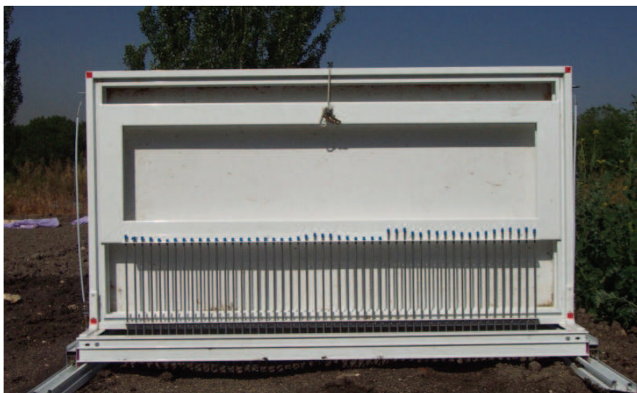
Fig. 1. Pin-meter used to measure soil surface roughness
