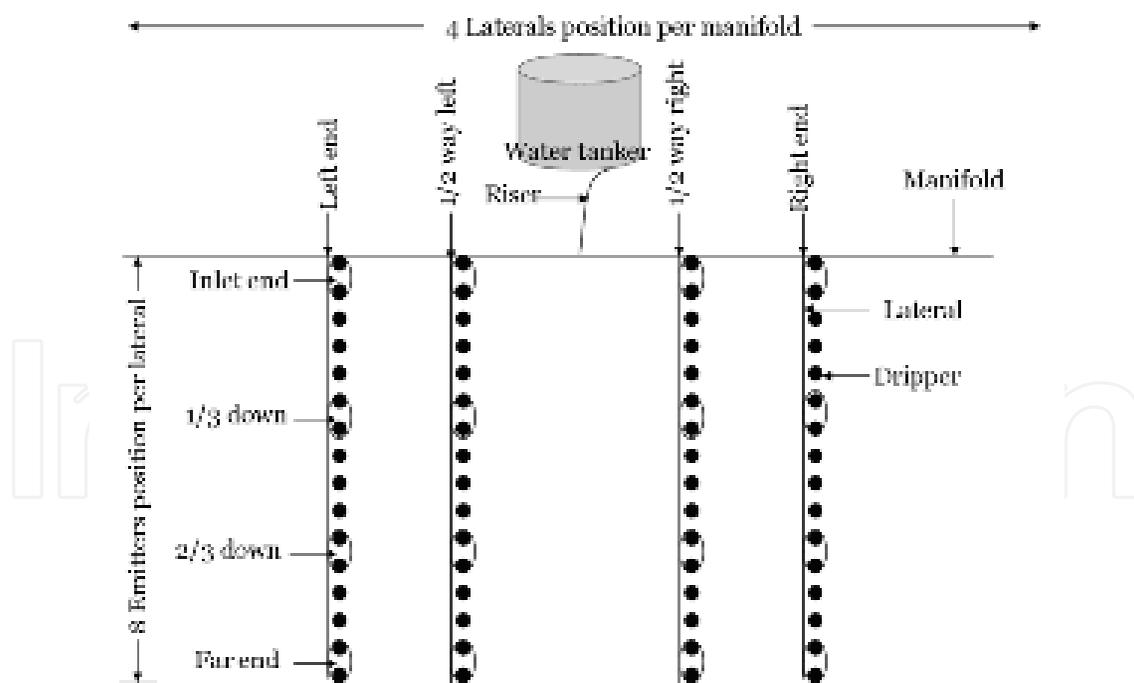
Total plot area 500 m<sup>2</sup>. Spacing between laterals = 0.75m and drippers = 0.3m, manifold and lateral length 20m & 25m
