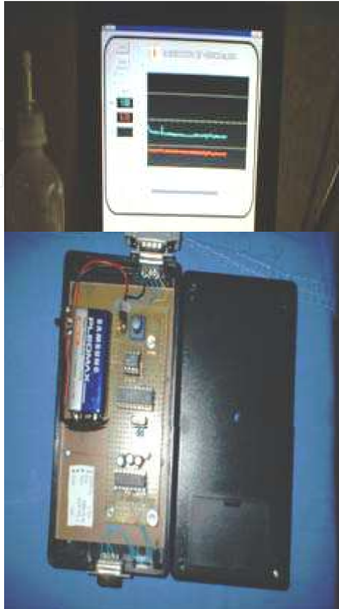
Fig. 2. Experimental Prototype by using PIC16F8767 Microcontroller and connection in the Hemodialysis machine
