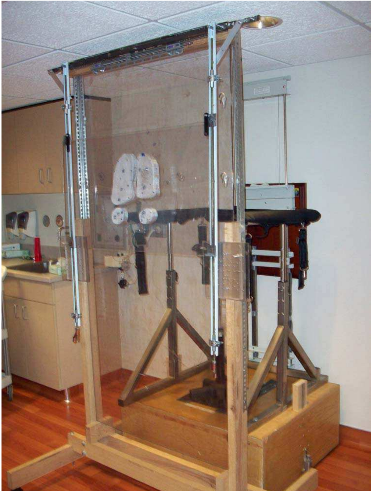
Fig. 5. Front view of mobile spoiler and blocking mechanism used in conjunction with TBI stand.
