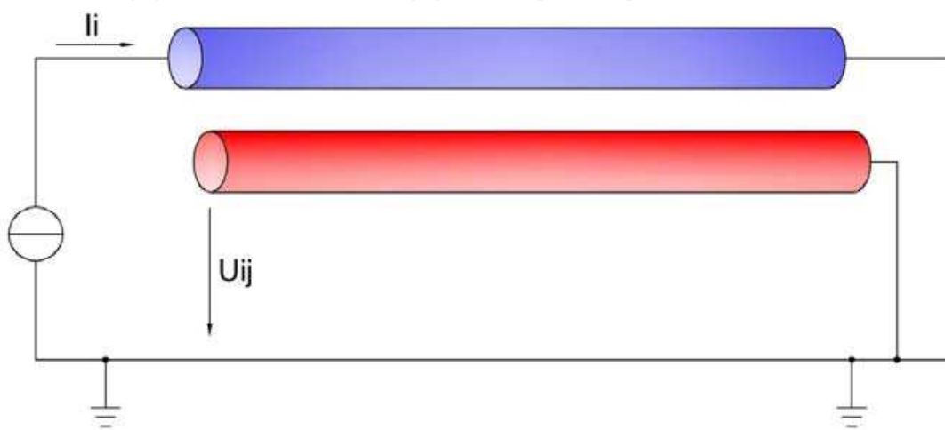
Fig. 5. Mutual impedance calculation
