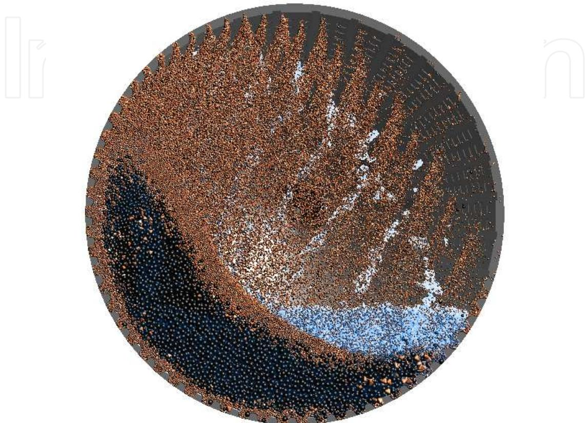
Fig. 7. A view with particle shapes at the mill center cross section.
