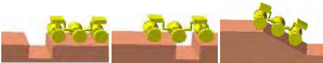
Fig. 10. Simulation for WMR with ADAMS and Contact model
