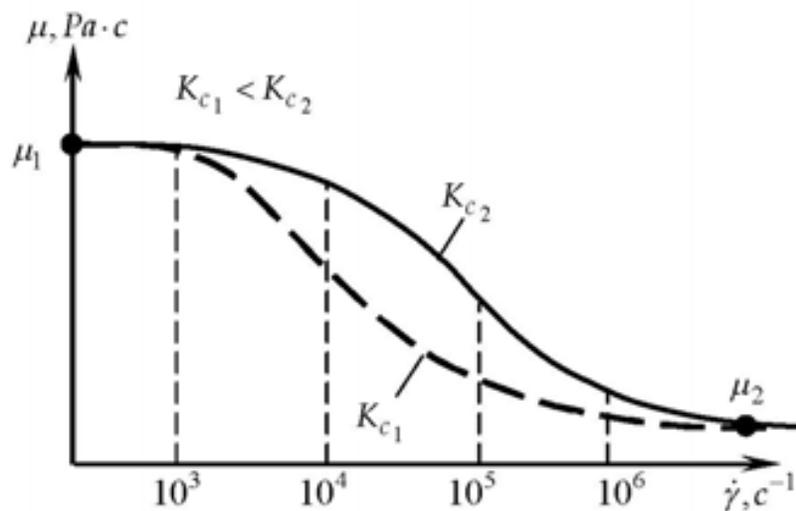
Fig. 7. Fundamental character of the non-Newtonian oils viscosity
