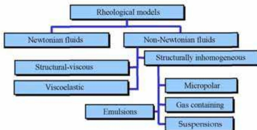
Fig. 5. Classification of rheological models of lubricating fluids
