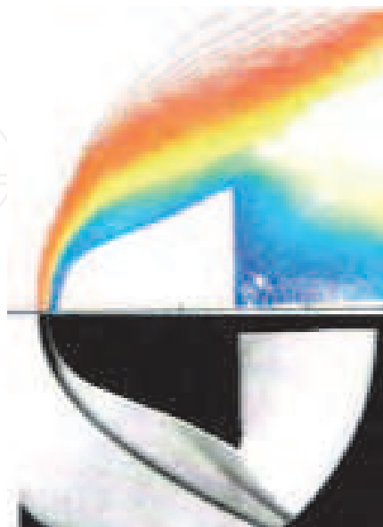
Fig. 4. Comparison between density contour and schlieren picture.
