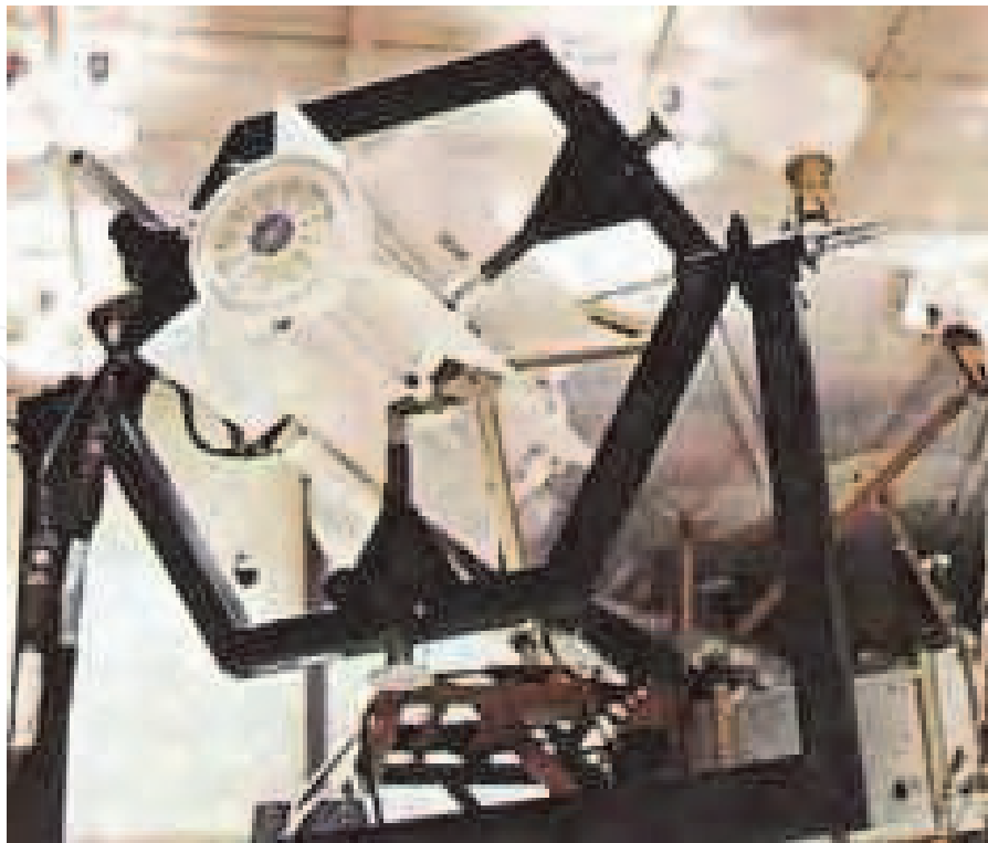
Fig. 12. SNAP-19s installed on Pioneer.
