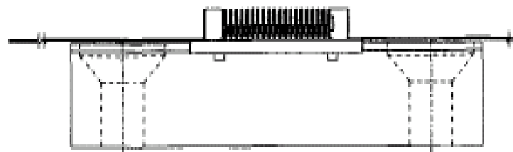
Fig. 16. 20 bar, 0.8 cm 2 array (1500 W/cm 2 ) mounted on a copper block. This design minimizes overall packaging costs.
