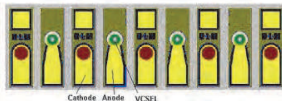
Fig. 14. Coplanar electrical access VCSEL array
