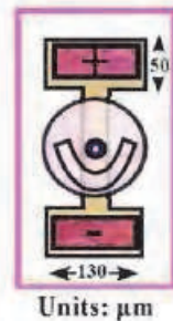
Fig. 15. Bottom-emitting Raycan VCSEL chip
