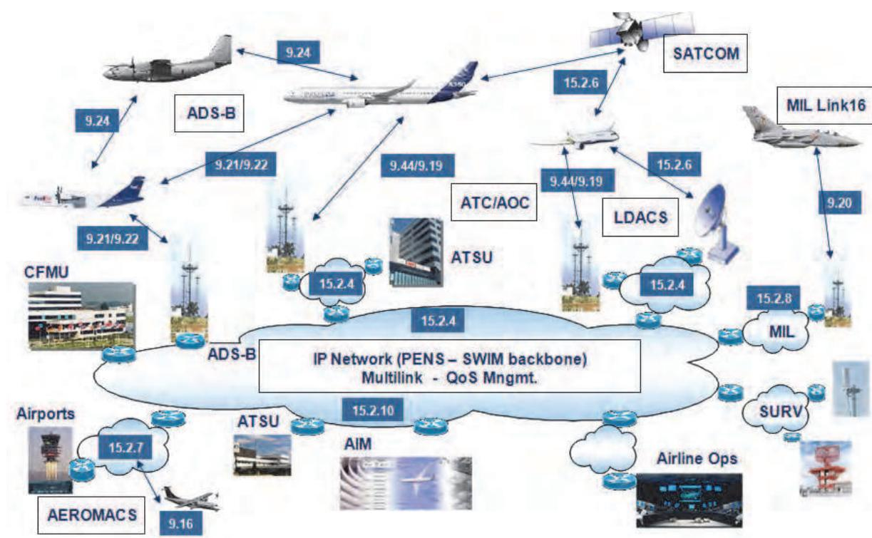
Fig. 3. Communication architecture.
