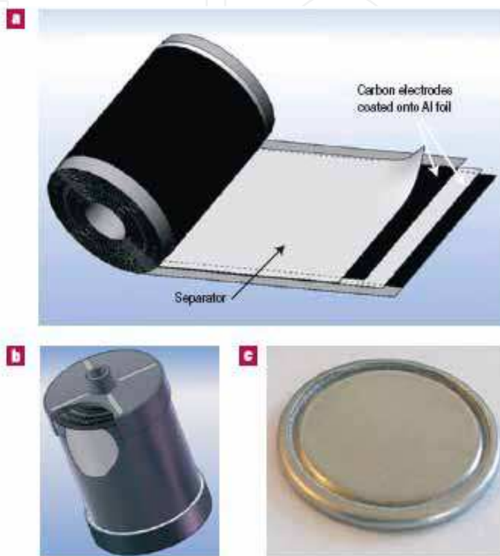
Fig. 9. a) Schematic representation of a double-layer spiral capacitor; b) assembled device (500 grams, 2600 F); Batscap, Groupe Bollorè; c) button cell (1.6 mm height, 5 F capacity); Y-Carbon.
