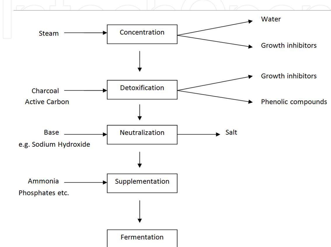
Fig. 1. General operations required after hydrolysis prior to fermentation.
