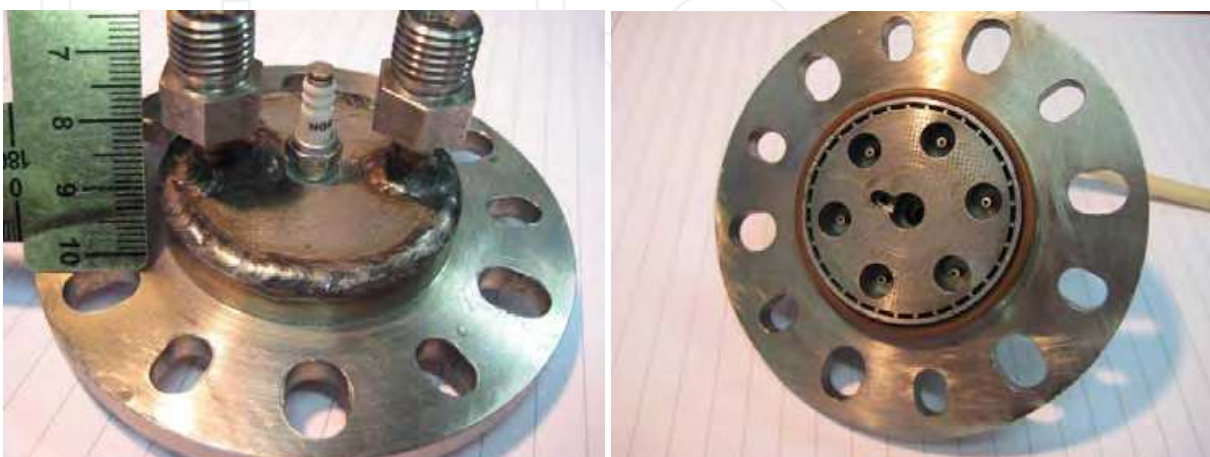
Fig. 12. Photography of mixing head.
