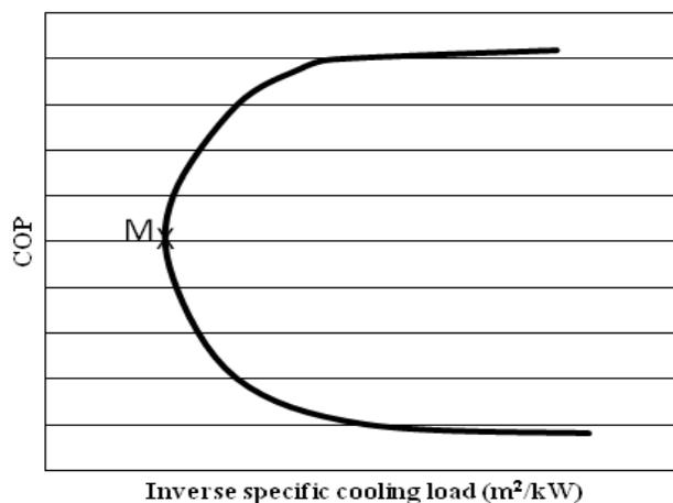
Fig. 2. Inverse specific cooling load versus the COP.
