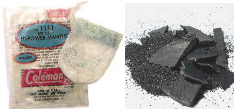
Fig. 1. Thorium dioxide with 1 percent cerium oxide impregnated fabric, Welsbach incandescent gas mantles (left) and \text{ThO}_2 flakes (right). Yttrium compounds now substitute for Th in mantles.
